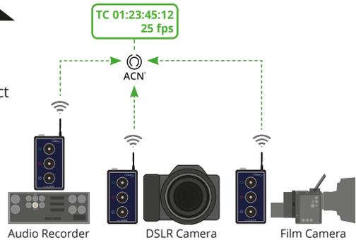
Timecode from an external source can now be sent from one device to other devices. This external source must be permanently connected to this NanoLockit via TC input or MIDI USB.
