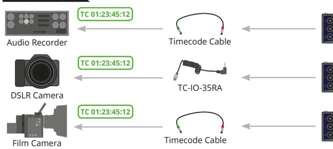
NOTE: Required cable depends on connected device. E.g. TC-IO for ARRI, LTC-Out/Epic for RED, LTC-Out for BMD, Canon, Panasonic, Sony. Please check our website.
