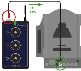
NOTE: Adjust the device menu settings to accept external timecode. Please check the manufacturer's manual.
