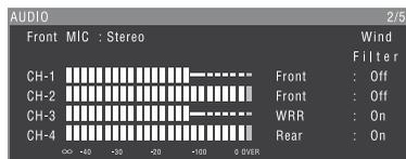
**CH-1/CH-2/CH-3/CH-4:** Audio level meters and input sources
