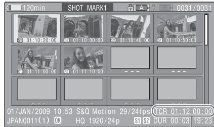
The properties of the clip appear at the bottom of the screen.
