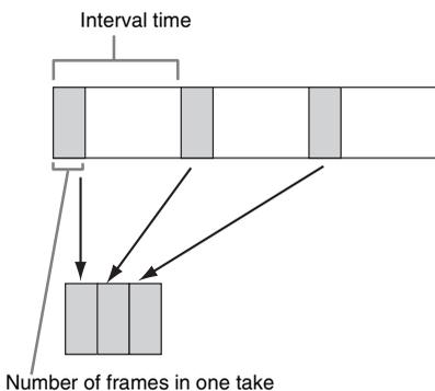
A pre-lighting function is available when Interval Rec is enabled. This function automatically turns on a video light before recording starts, which allows you to record pictures under stable light and color temperature conditions.
