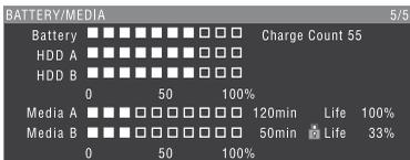
**Battery:** The remaining battery capacity
